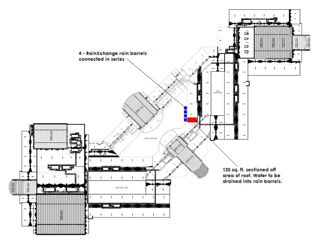
Figure 10: Proposed rain barrel layout
