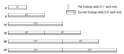
Modular section lengths offer standard 4'0", 8'0" and 12'0" support spacing that aligns with grid ceiling systems.
