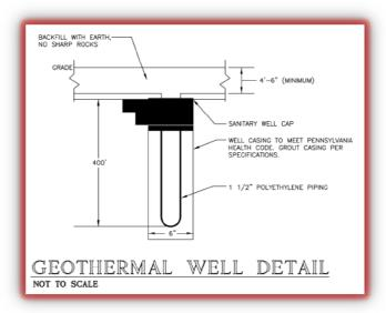
Figure 6: Geothermal Well Detail
