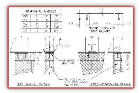
Figure 7: Steel Beam CMU Wall Bearing Details
